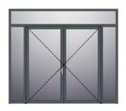
Glazed double hinged door with top and side panels, in aluminium or as steel tube construction.
