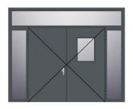
Double steel plate door with glazing and glazed top and side panels.
