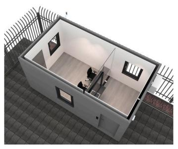
Example of interior design: use of a glazed security partition wall, including a transaction window with transaction drawer and intercoms. The first room is for the guard staff and the second one can be used for performing security checks on individuals.
