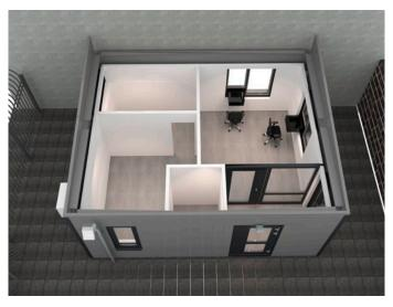
In this example, the guardhouse consists of 2 modules. With a total of 5 rooms (guard room, control room with 2 interlocking doors, technical room, sanitary facility and kitchen area), it is suitable for use by a whole team. As an option, a mono-pitch roof can be installed, with adaptations to suit the local conditions.
