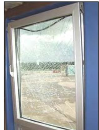
**SECURON<sup>®</sup>** successfully tested with 100kg explosive; reflected pressure: 0.87 bar.
