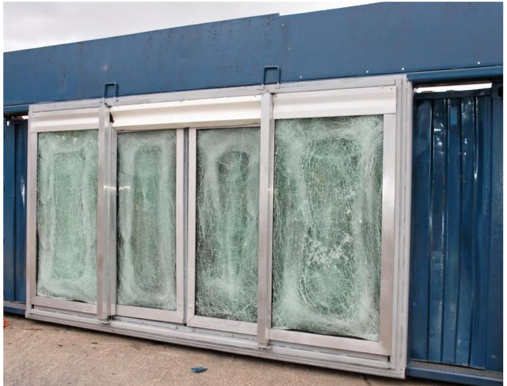
Double sliding door with side lights. Size: 4.405 x 2.530 m with 500 kg charge successfully tested. The whole door withstand the enormous blast wave of about 24 t pressure / sqm.
