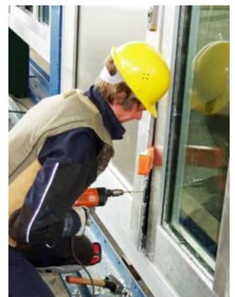
In the forced entry tests in accordance with European standard DIN EN 1627-1630 electric tools are used from the resistant level RC4 (or WK4). The above photo shows the examiner of a renowned German test institute, trying to drill out the lock side of the SÄLZER aluminium door **serie S6es** by a power drill.
